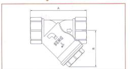
Female/female threads and inspection plug. Body in brass.
