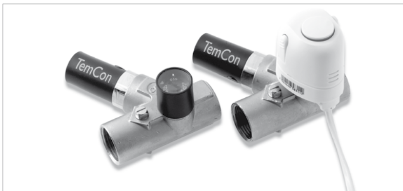
TemCon + fem./fem. valves with scale by-pass and actuator by-pass respectively both of them with built in isolation ball valve.
