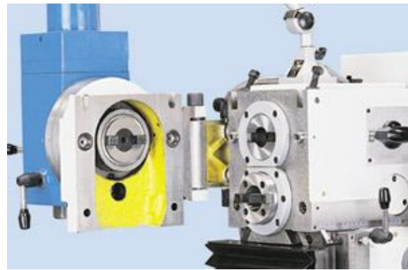
Swivel arm moves the vertical cutter head for horizontal milling
