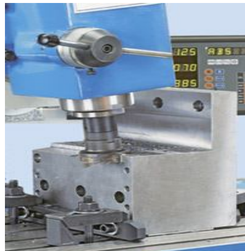
Infinitely variable vertical cutter head with a swivel range of \pm 90^\circ
