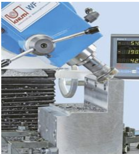
Infinitely variable vertical cutter head with a swivel range of \pm 90^\circ
